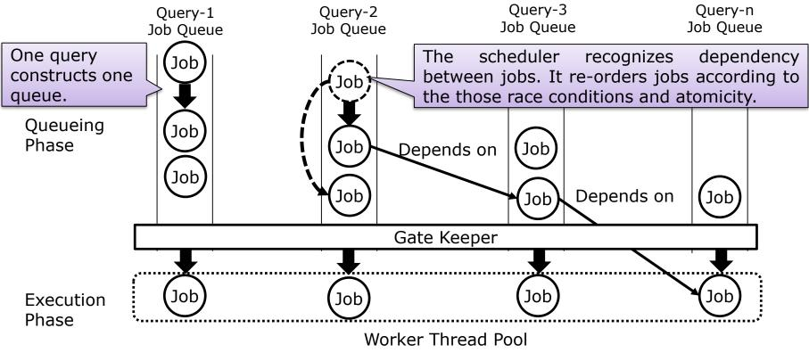
In the immutable query model, DB engine can schedule threads perfectly without synchronization lock.
