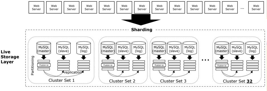
Data mining process including JOIN operations is carried out by replica DBs that are replicated from the master database asynchronously.
