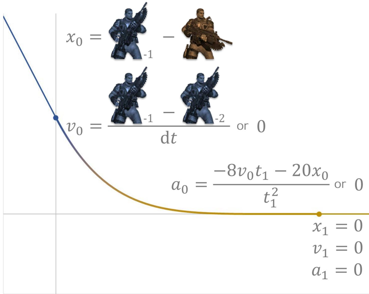
$$A = -\frac{a_0 t_1^2 + 6v_0 t_1 + 12x_0}{2t_1^5}$$
