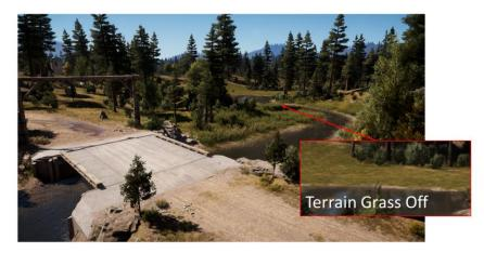
We place grass instances each frame with a compute shader that samples the terrain material type, height, color and normal.
