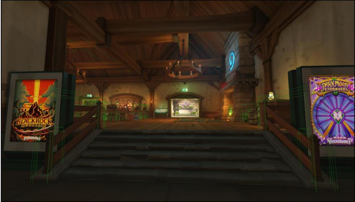
All the objects in the map, the floors, the walls, the chairs are objects that are enclosed in axis aligned bounding boxes. This is done to accelerate collision detection.
