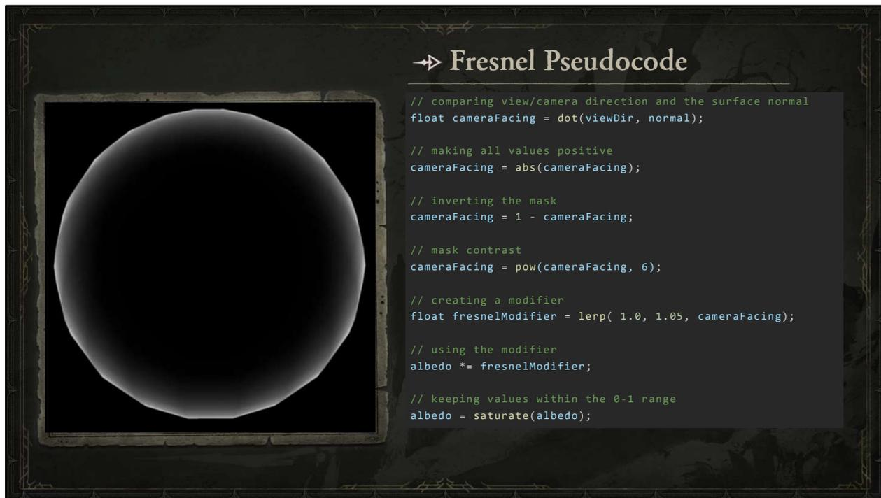
For creating the Fresnel effect, we want to compare the view direction (which is where your camera is pointing, and the surface normal. So to begin, we're looking at a visualization of the normal.
