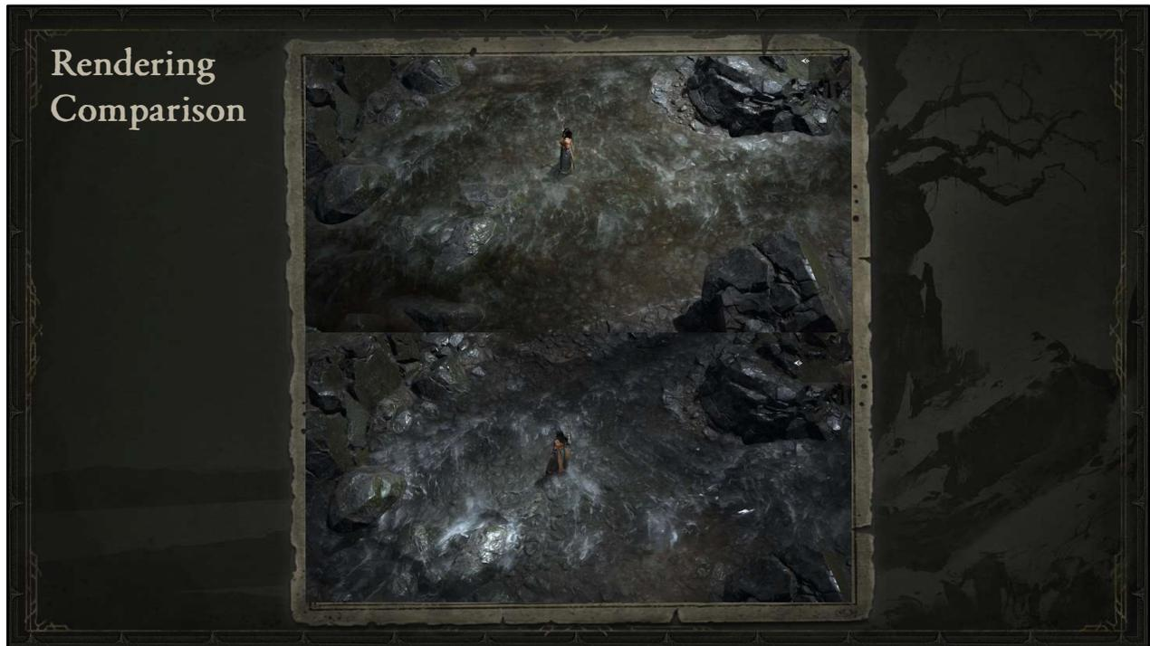
Here you can see a comparison with Gbuffer water on top and forward rendered water on the bottom.
