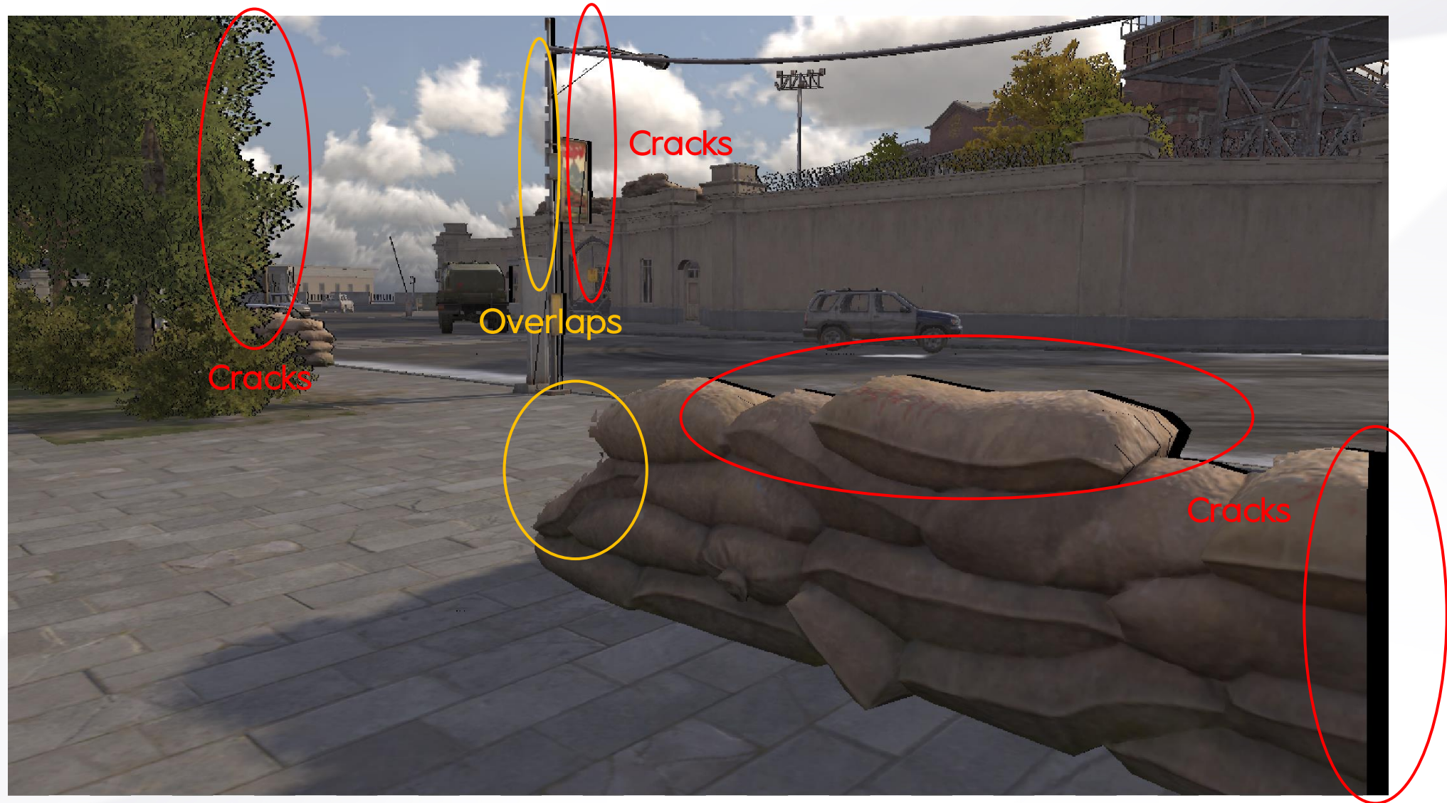
Crack and overlap of per-pixel reprojection
