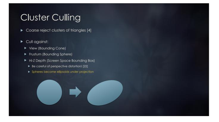
This approach allows for us to coarse reject entire clusters of triangles prior to the per triangle culling pass. Additional per cluster tests include bounding sphere vs frustum, and testing the bounding sphere's screen space bounding box against a Hi-Z depth pyramid. Be careful that you account for perspective distortion, as spheres become ellipsoids under projection.
