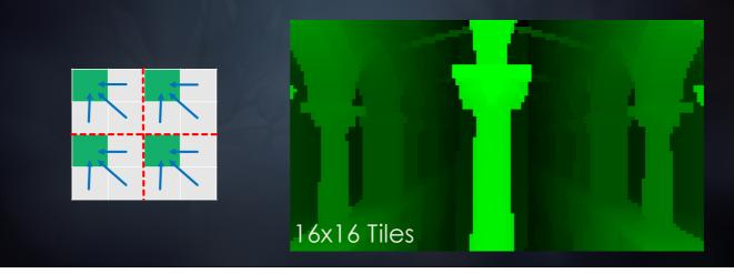
Another available triangle culling approach is to do manual depth testing. However it is worth noting that directly reading depth for cluster or triangle culling is extremely scene dependent due to availability, and the quality of occluders at any given time. The general technique is to take the depth buffer and perform an LDS optimized parallel reduction [9], storing out the conservative depth min or max value for each tile.
