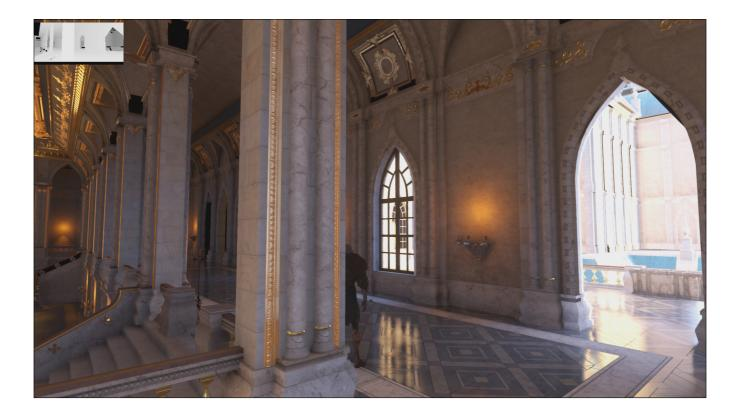
This image shows Solas behind a pillar, and the results of the CPU rasterized occlusion buffer in the top left. Using this buffer, a Hi-Z pyramid was constructed, and the triangles for Solas are being depth tested against the appropriate mip level in this texture.
