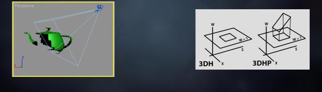
On average, 50% of a mesh will be culled from backface. So we need a test which is as cheap as possible. One of the cheapest tests is the one described in this paper [3], using the determinant of a 3x3 matrix with homogeneous coordinates [2]. This technique avoids clipping and projection, which includes ¼ rate reciprocal instructions coming from the perspective divide.
