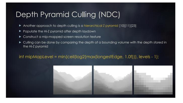
Another approach to depth culling is a hierarchical Z pyramid [10][11], which starts at the resolution of the depth buffer, and goes all the way to a single pixel. The first level of the pyramid is populated after depth laydown, similar to the depth tiles method. After which, we populate the remaining mip levels in the pyramid through a custom downsample pass.
