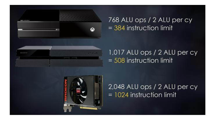
Finally, if we divide the number of ALU ops per triangle by the number of ALU ops per clock, we get a final instruction upper limit that we have to cull a triangle with, and still beat the fixed function primitive setup and scan converter.
