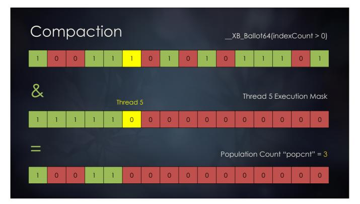
Taking ballot further, we have this example showing thread 5. Before thread 5, we have three other threads that are valid, so we want to calculate the value 3 for thread 5's output slot.
