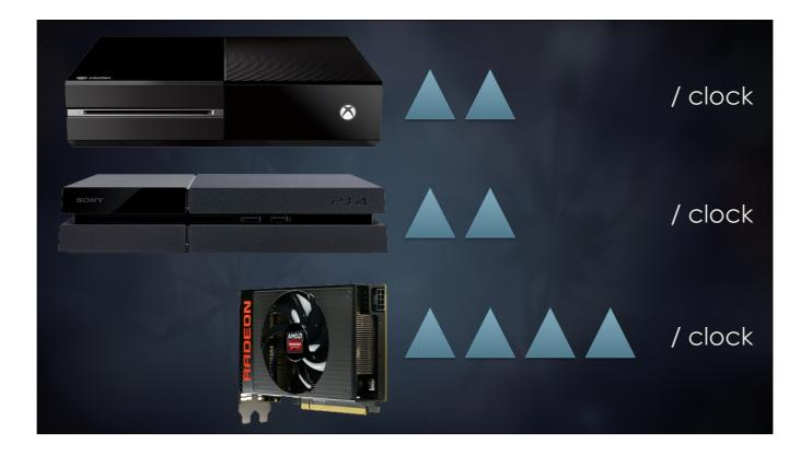
Lets break down peak triangle rate for our target platforms, and prove how we can beat it. Both Xbox One and PlayStation 4 have 2 shader engines, where each can issue 1 triangle per clock. Newer AMD GPUs on PC have 4 shader engines, so a total of 4 triangles per clock.
