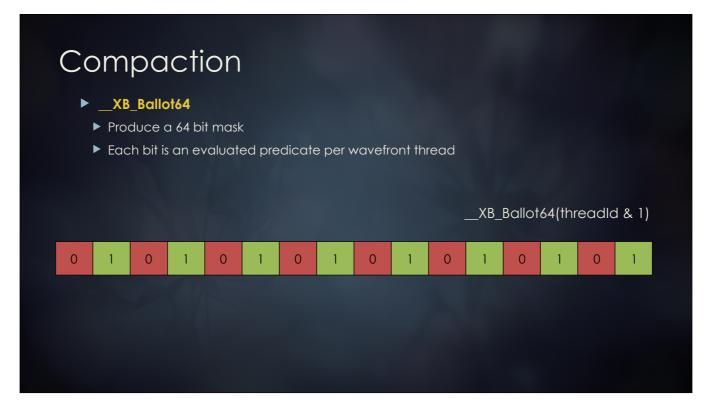
The first thing to mention is a compiler intrinsic known as ballot. Ballot can be used to construct a 64 bit mask where each bit is an evaluated predicate per wavefront thread. For inactive threads, based on the execution mask, the bit will be 0 for these threads.
