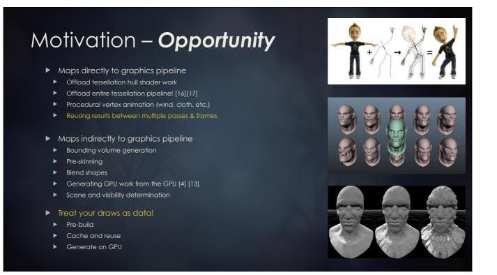
Compute shader mesh processing opens up opportunities for more efficiently supporting a variety of high fidelity features and improvements. Better yet, by reusing post-shader results between multiple passes, and doing less draw setup work on the CPU, there is increased optimization potential.
