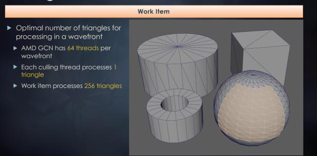
Lastly, we have a work item, which represents a subset of triangles in a batch that will be processed by a compute shader wavefront.
