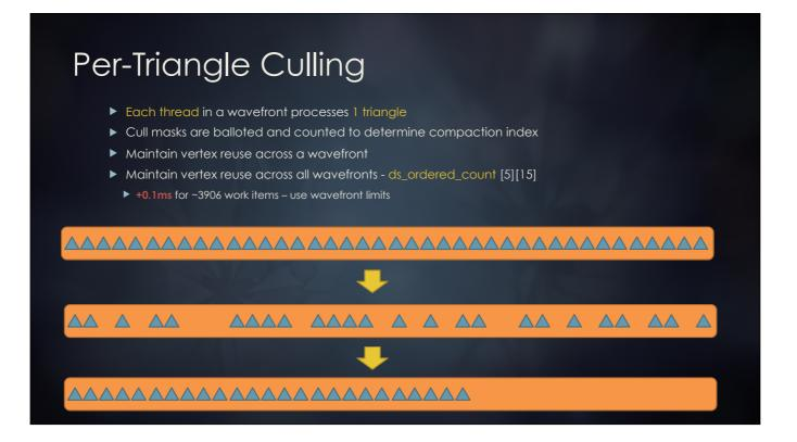
As mentioned already, each thread in a wavefront processes 1 triangle. Various culling operations are applied, and the surviving triangles across a wavefront need to be counted to determine the compaction index, or, the location in the resultant index buffer where the surviving indices will be written. This step is important for maintaining vertex reuse across a wavefront.
