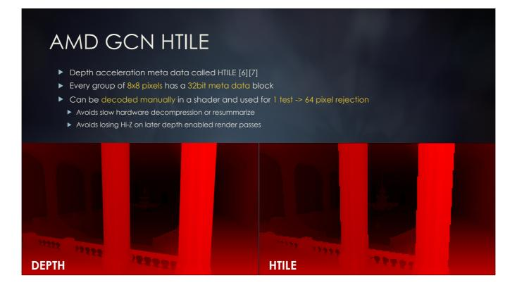
GCN has a depth acceleration meta data called HTILE [7] which accelerates regular GPU depth operations. Every 8x8 group of pixels has a corresponding 32 bit meta data block. While this meta data accelerates regular GPU depth operations, it can be decoded manually in a shader and used for early rejection of 64 pixels with a single test, or for any other relevant purpose.
