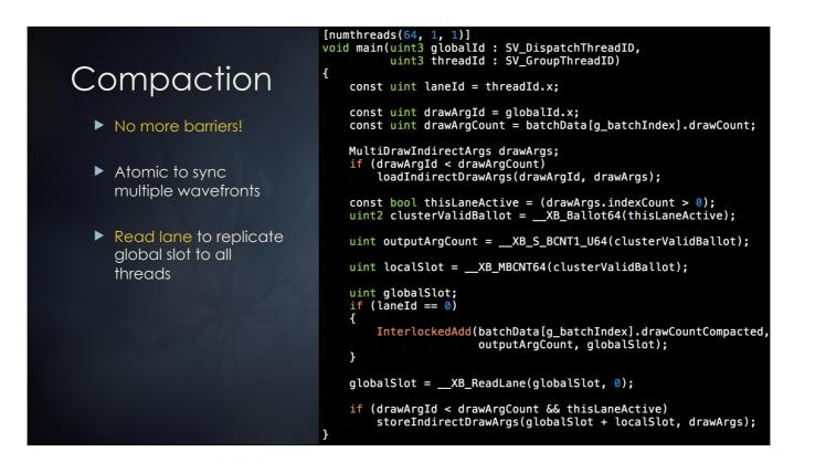
The GCN optimized compaction shader looks like this. We no longer have any barriers. In order to compact across multiple wavefronts, we have a single atomic operation per wavefront that reserves the output space for all the surviving draw calls across each wavefront.
