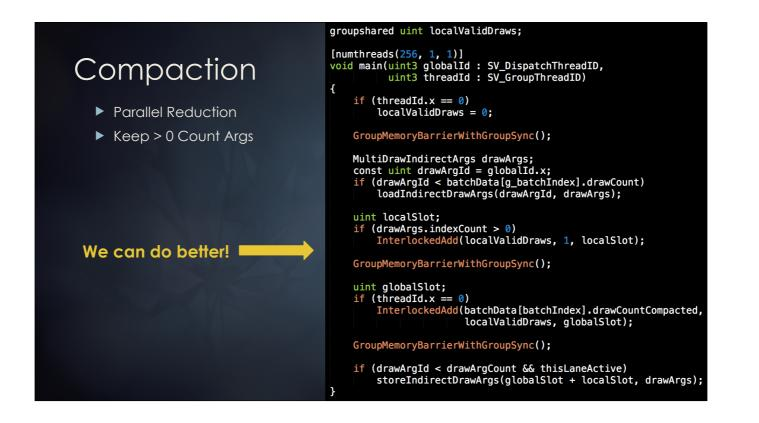
A cross platform approach to draw compaction is to do a parallel reduction with atomics in group shared memory. Each thread loads the indirect arguments for a draw and determines if the draw is worth keeping. A barrier allows all threads to complete and then the first thread in a group allocates output space for the surviving draw args.
