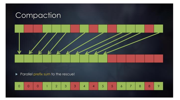
The issue with optimizing the compaction is that each thread needs to write in a contiguous range, so using the thread id as the index wouldn't give us this, and we want to avoid global synchronization like the previous compaction algorithm.
