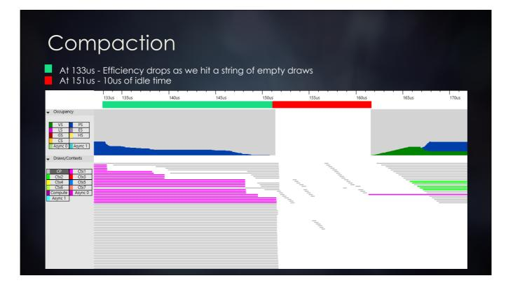
The grey draws in this GPU capture are empty draw indirects. At first, the command processor (CP) cost is hidden by in-flight draws. Around 133us, the efficiency drops as we hit a string of empty draws. At 151us, we suffer around 10us of idle time.
