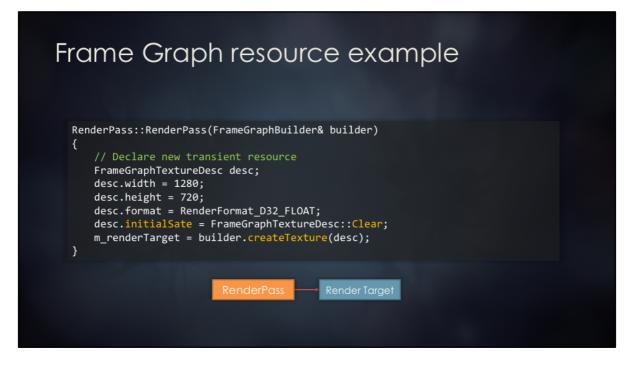
Simple dummy render pass that produces a render target resource.
