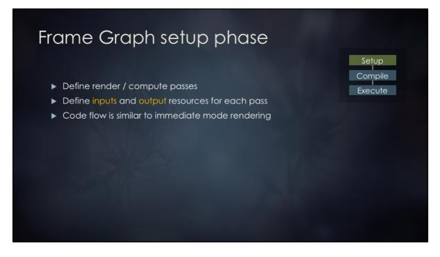
Flow is similar to IM rendering, but we are not generating any GPU commands during this phase. Just building up the information about rendering operations for the frame. All resources are virtual during graph building. Render pass inputs and outputs are declared using virtual resource handles.
