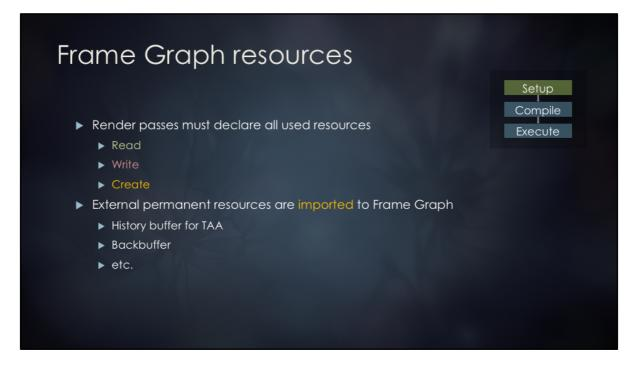
Some render passes may have effects that are not visible to FrameGraph (for example data read-back from GPU). Such passes are explicitly marked as having side-effects.
