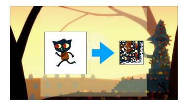
Here's a peek at the result of the process outlined in this talk. We're taking a large sprite that has lots of empty space around the edges, but also within its trim-able area. It also has quite a bit of redundant areas of the same colour.
