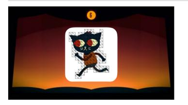
The downside to this is that our mesh density has gone up a bit - each vert is like 18 bytes. However, the additional mesh cost is much lower than the savings we get by storing fewer pixels of texture data.
