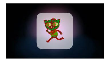
Note how the green blocks are largely flat areas of colour, but non-flat blocks exist, such as near the waistline of Mae's shirt - it's green because another frame elsewhere in the sequence has a copy of the pixels, so only one copy is needed.
