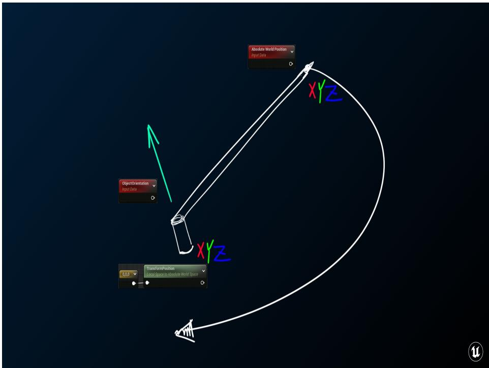
To draw that out, we need to rotate this dial (at each vertex), from the worldspace origin of the primitive, around the axis ObjectOrientation, by the amount we calculated earlier.
