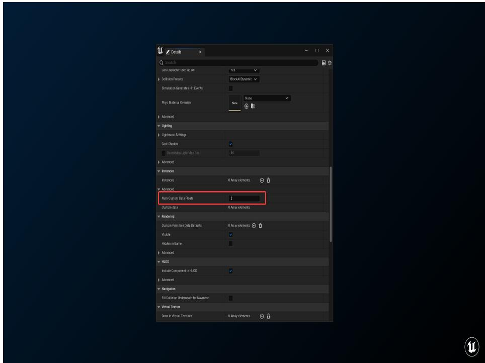
On the `InstancedStaticMeshComponent` I need to tell the engine that I'm going to pass in some per-instance data with the `.NumCustomDataFloats`. This is going to be the "SwayAmount" and the "LinePercent". You can ALSO set `CustomPrimitiveData` on `InstancedStaticMeshes`, but they'll be applied to all the instanced in the component.
