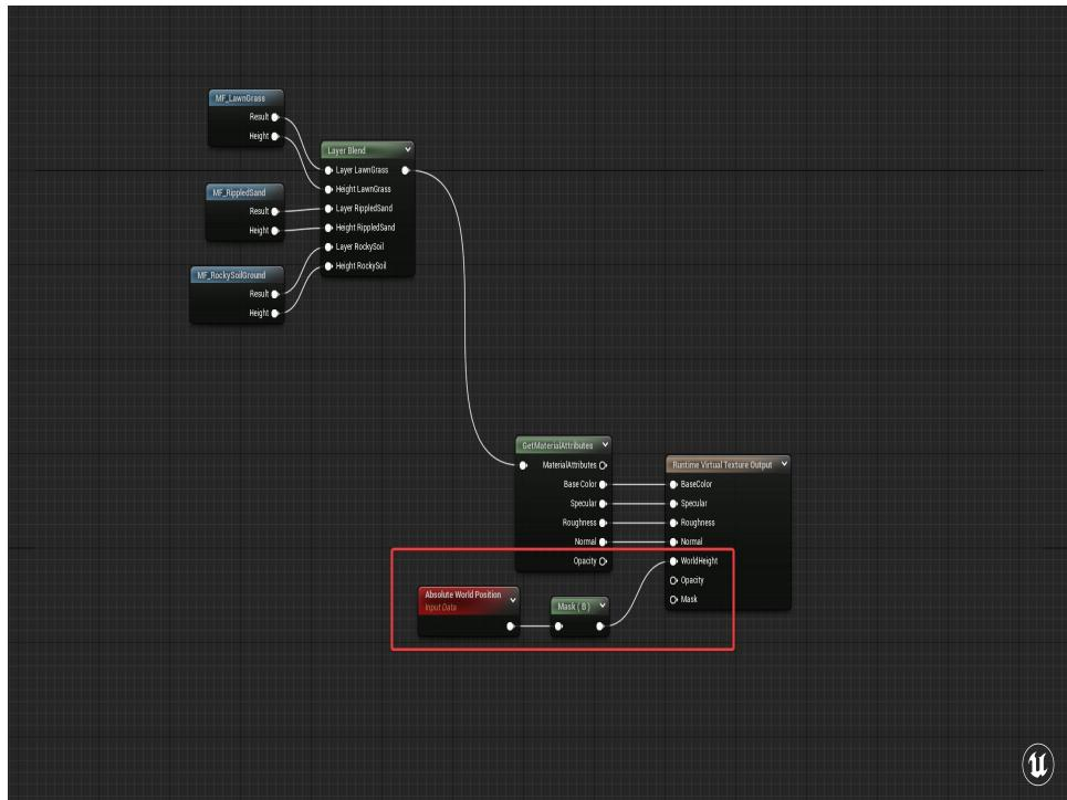
Jumping back to the Landscape material, all I'm doing here is taking the Absolute World Position of the landscape, masking it to the B component (or Z) and passing that into the World Height input of the Runtime Virtual Texture Output Node.
