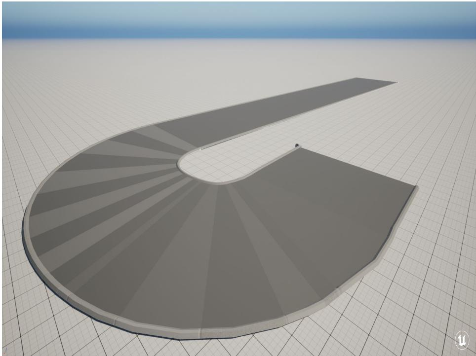
Most recently, I used it to pass in a “Bendiness” parameter to a spline mesh race track maker. As the start and end tangents of the section diverge, I lerp in that little stepped pattern in order to let players know that the track is curving.
