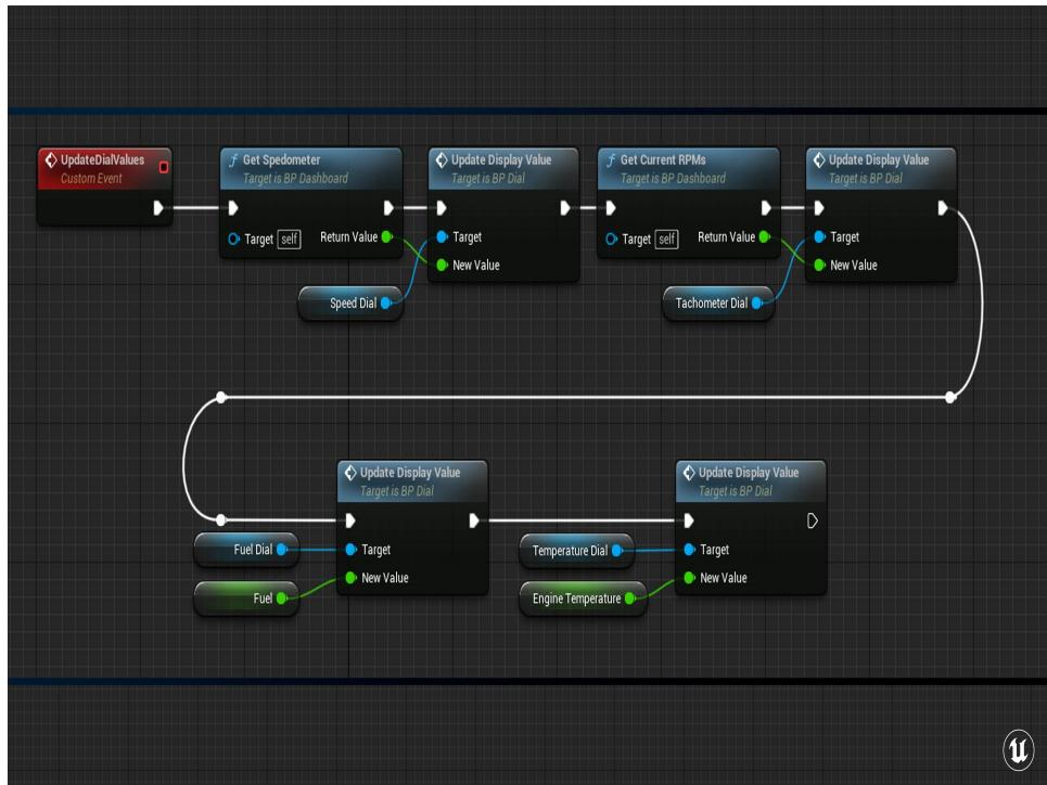
Then, in the dashboard Blueprint that handles all of the dials, we pass in the appropriate values for each of the different dials. RPMs to Tachometer, Speed to Speedometer, etc. This gets called every frame to keep those values up to date.
