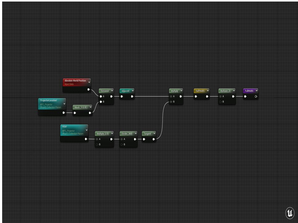
Now that we have the size of the opposite side of the triangle with half the FOV, that means that the full size of the projected texture is double that.
