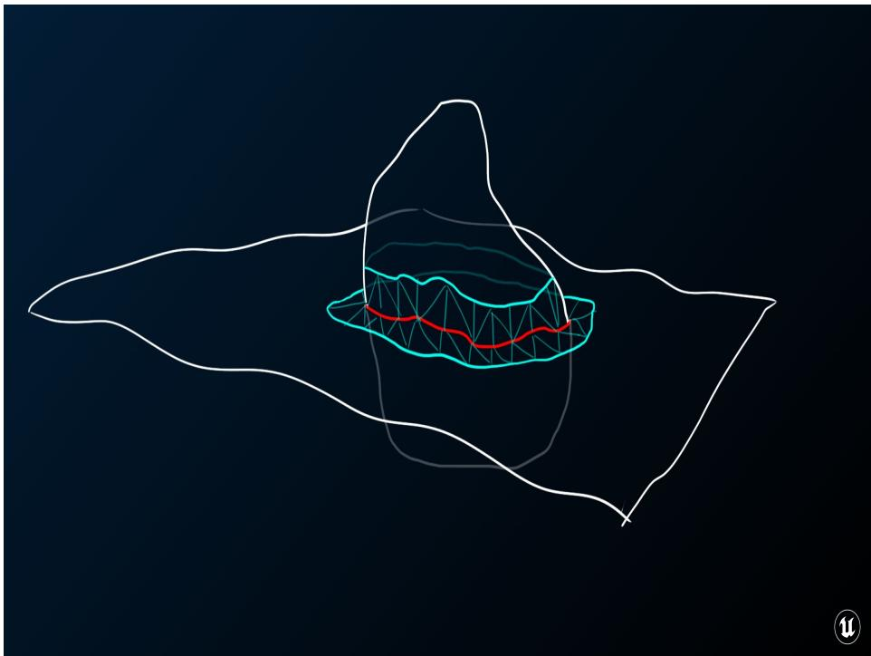
For that technique, you export part of your landscape and your whole rock to Houdini (or now in the Unreal Engine you can do this with the Houdini Engine directly in your application), determine the intersection between the two, create a little skirt of geometry with some alpha around the edges, and apply the landscape material (or a similarly-shaded purpose-built material) to the skirt.
