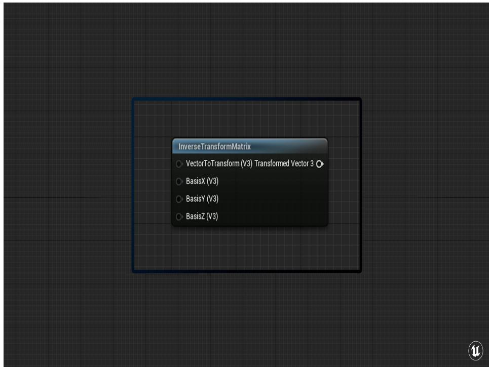
Unreal doesn't have the ability to construct and transform vectors into arbitrary spaces though, but it does have the `InverseTransformMatrix` material function, which does the same thing when you pass in vectors that define the space.
