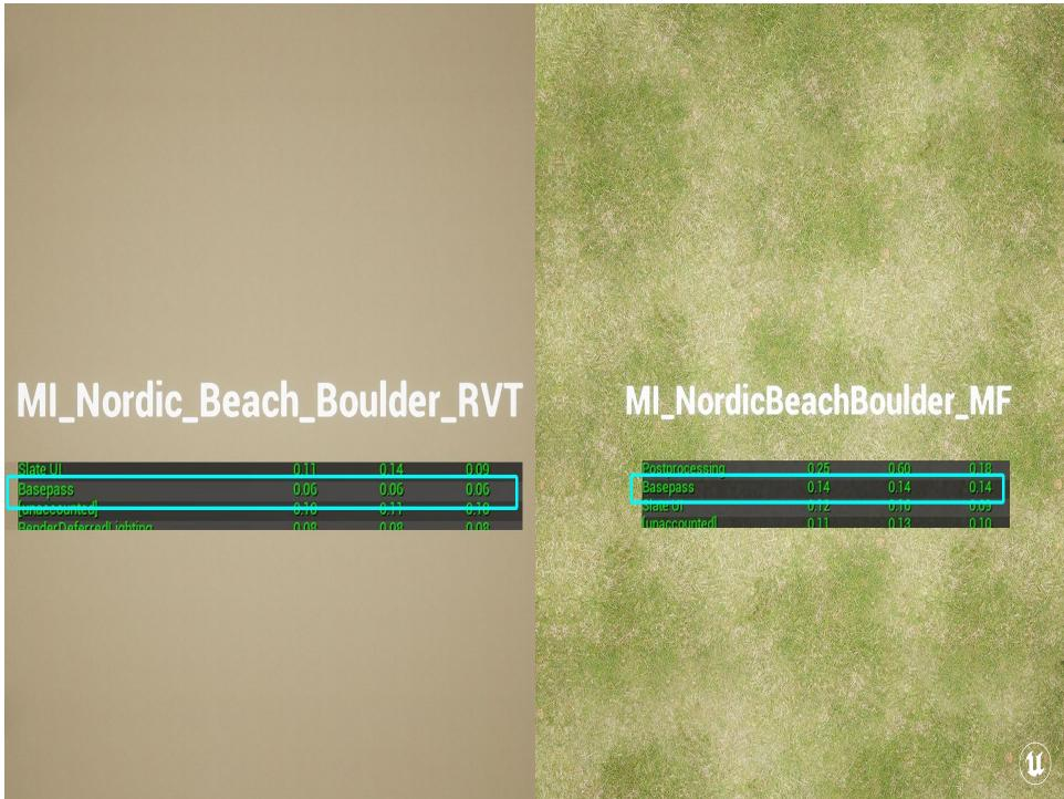
To test the performance differences between this technique and some alternatives, I created a full-screen quad and swapped between two materials: the base RVT blending material and one that has a material function that blends all the material layers together. Swapping back and forth between those two showed a roughly .1ms difference in the base pass cost on the GPU.
