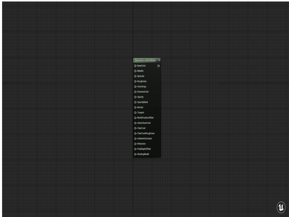
As a quick aside, in Unreal there's the a concept of “Material Attributes”, which is a giant struct of all possible material inputs that get passed around the graph, and it's really useful for organizing large material graphs or breaking up complex operations. So that's what that GetMaterialAttributes block was in the previous graph.
