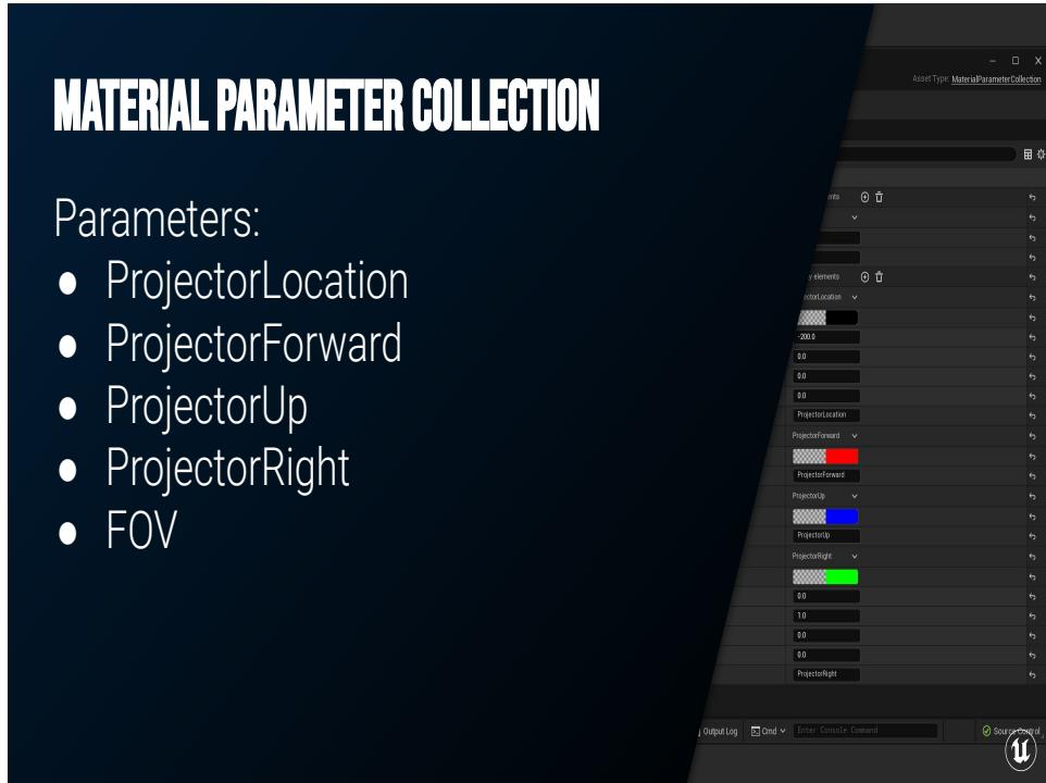
We can set up a Material Parameter Collection called MPC\_Projector, and set up four vector parameters for location, forward, up, and right vectors. There's also a scalar parameter called FOV.
