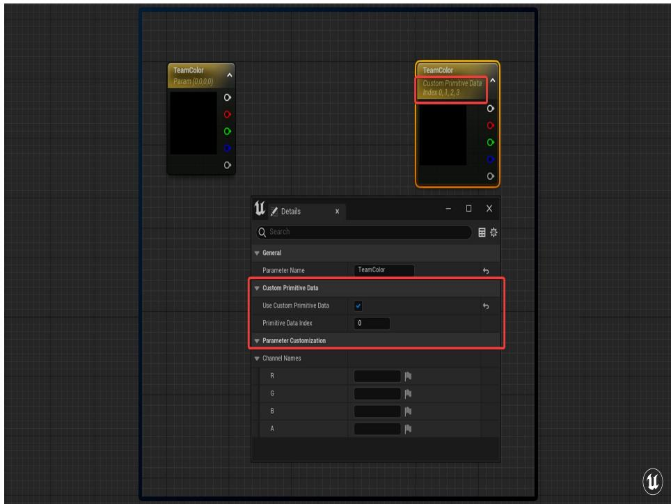
The first step is rather trivial! On the material, I have a vector parameter called TeamColor. I just check this checkbox that says “Use Custom Primitive Data”. This pipes into a mask that overlays the jersey barrier’s base material.
