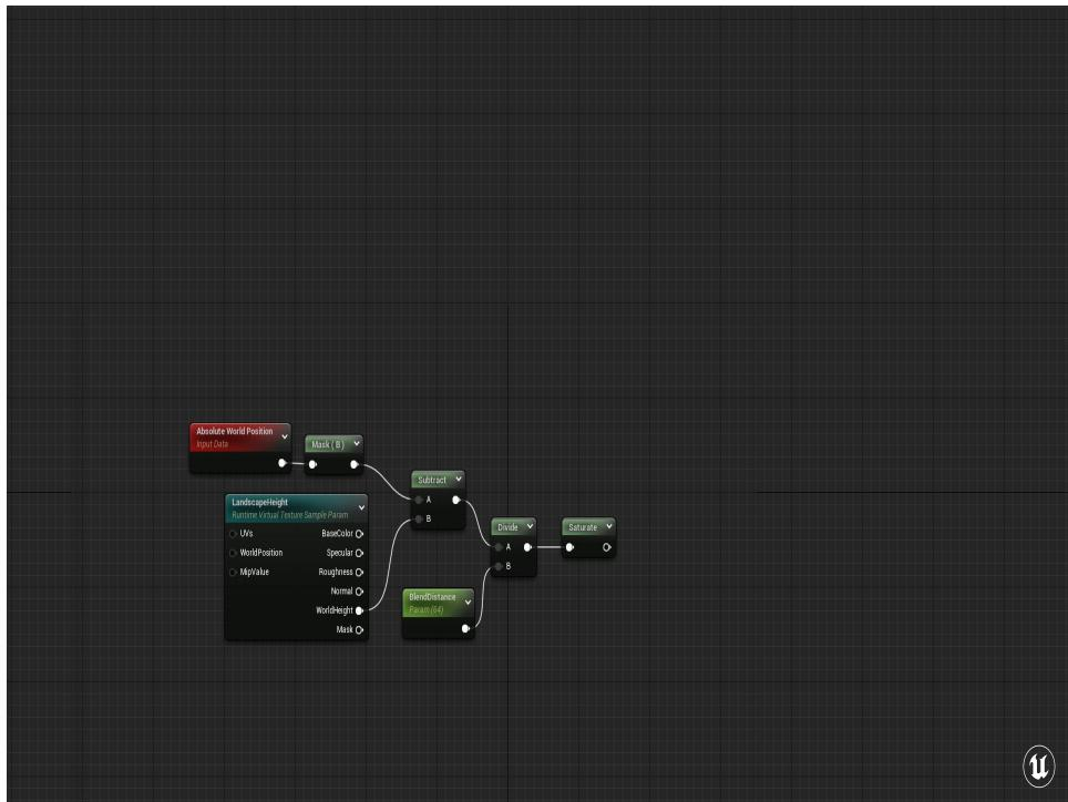
Then saturate the result, to keep it between 0 and 1. A saturate is just like a  $\text{Clamp}(0, 1)$  but is less computationally expensive or even free depending on the graphics hardware.
