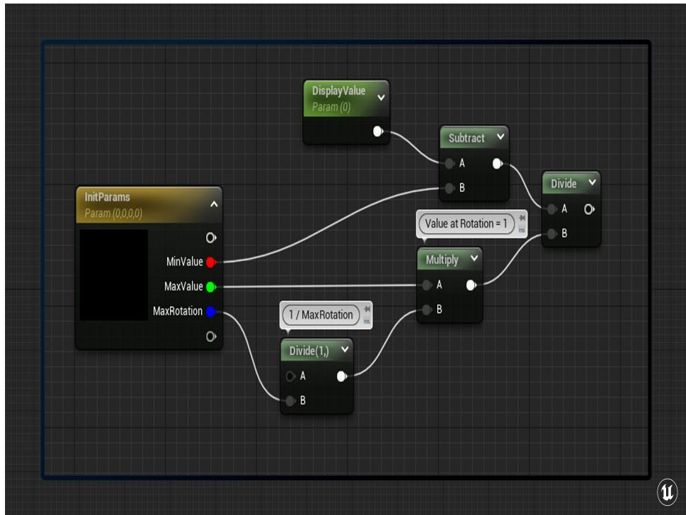
We're going to rotate the indicator with World Position Offset, or the Vertex Shader. And to do that we need a rotation value between 0 and 1. Sort of!
