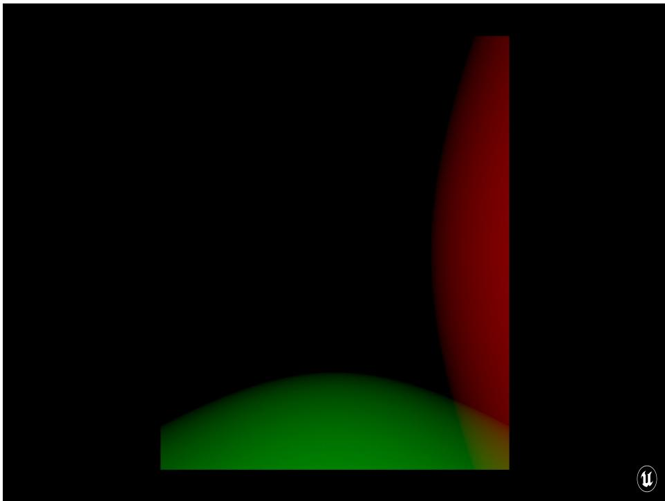
Except not, because we can't just normalize the transformed vector against itself. The PixelProjector vector isn't a unit vector, it's got magnitude equal to the distance between the projector and the pixel. And at that, this doesn't account for the FOV of the projector. This vector wouldn't give us a 0 to 1 space until it reaches full down or fully right, which isn't helpful for us at all.
