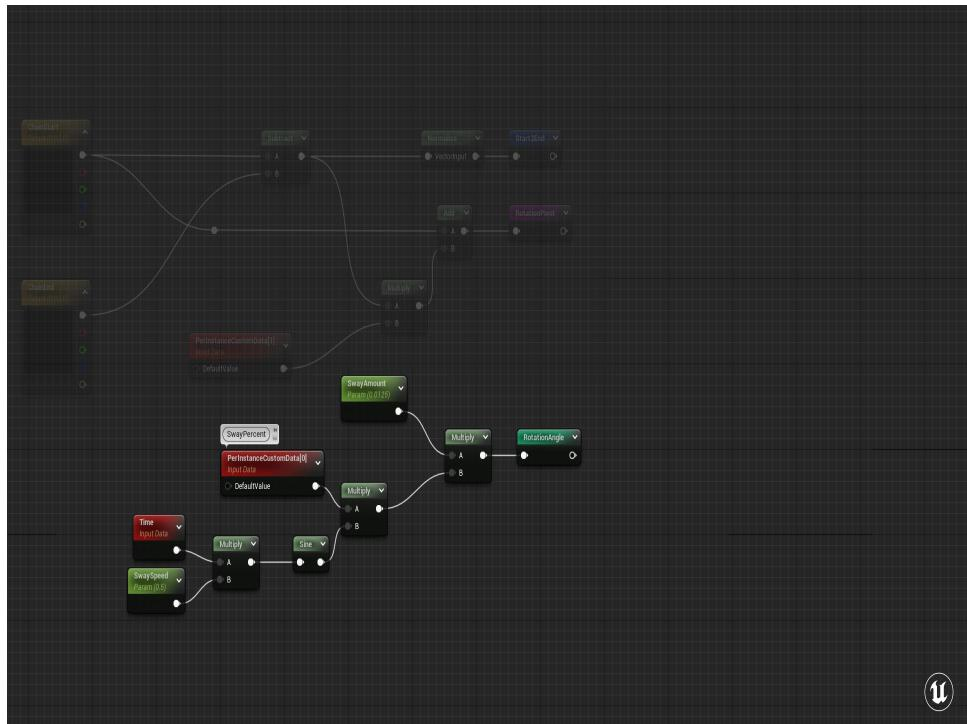
And for the rotation angle, I'll multiply the SwayPercent by the Sine of Time, then multiply that by a total SwayAmount that limits the extent of the rotation
