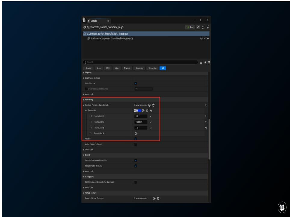
So all I need to do is add three custom primitive data floats, and the engine knows that the first one is Red, then green, then Blue. If I want to save myself one float worth of memory, I can skip adding the four one for the alpha channel because we don't use that in our material. If we added additional custom primitive data parameters we'd need to add the alpha channel, though, because these indexes are order dependent!
