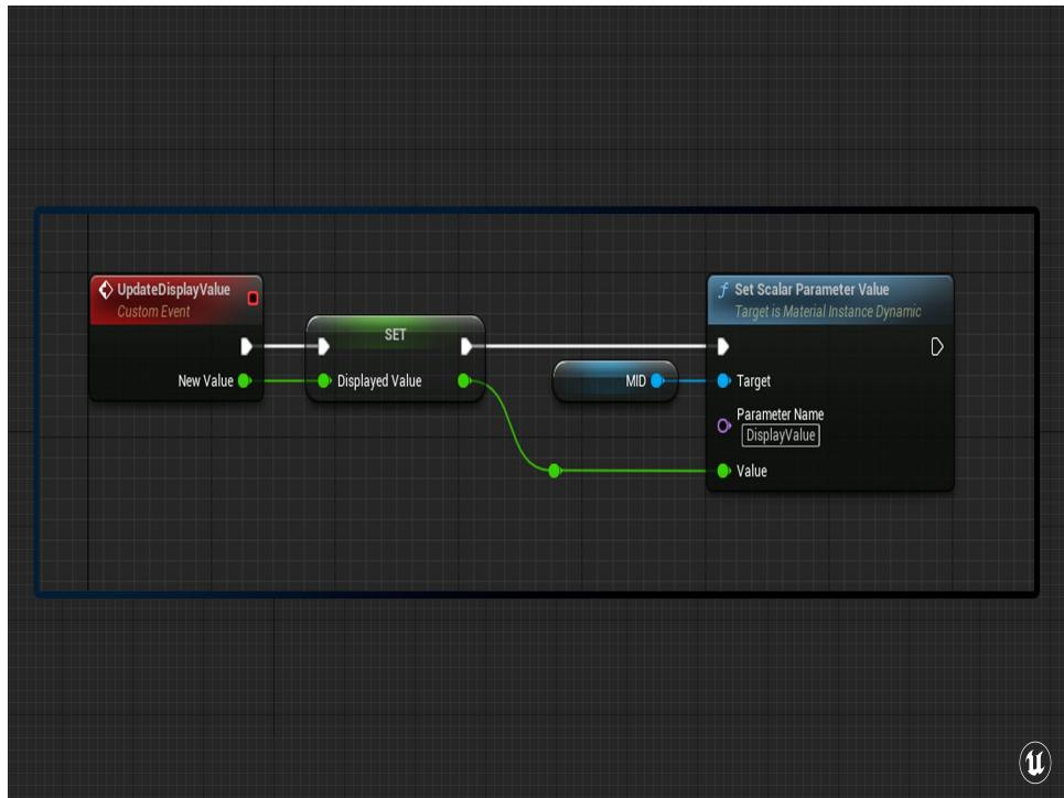
Then this blueprint has a function that passes an input “Display Value” into the material instance as well. All these dials are going to use the same parameter name, `DisplayValue`, because they don’t care what they’re displaying.
