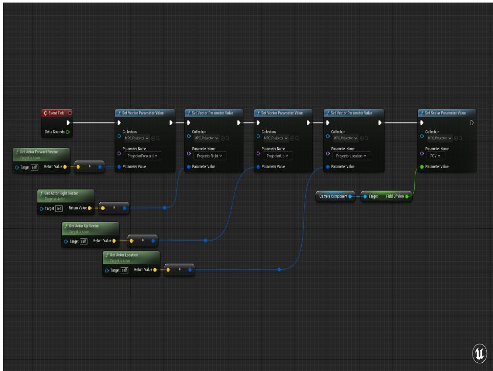
I create a Blueprint based off the Camera actor called BP\_Projector. Every frame it uses Set Collection Parameter pointing to that MPC we created to pass in its location, forward, up, and right vectors, and its FOV. We're taking all our known information and sending it along to the material.
