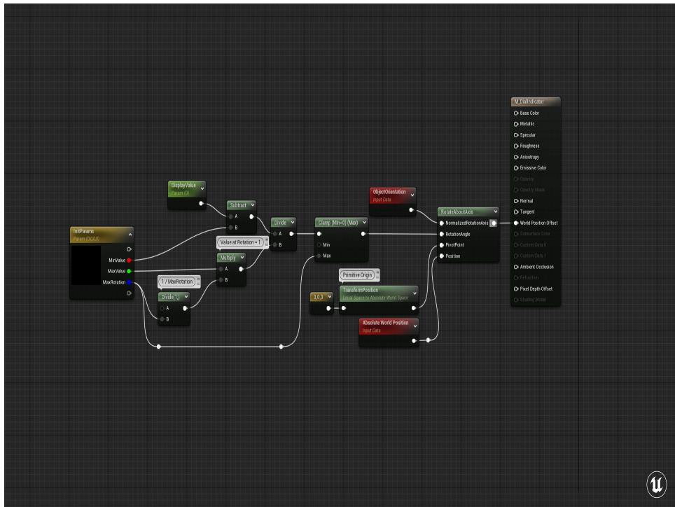
Then we just pass that output of the RotateAboutAxis node to the WorldPositionOffset input of the main material node. For Unreal, we run a standard vertex shader for each vertex that puts it at the position encoded in the geometry, and we have the option to offset that position in worldspace. That's all we're doing here!
