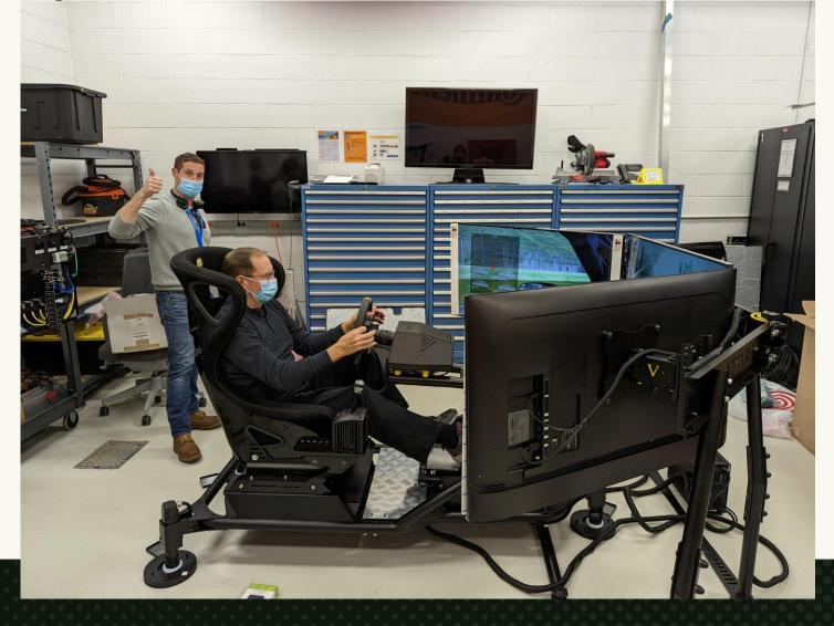
Video of driving simulator used to showcase use cases of Wrong-Way Driver Detect and Alert system being developed by Continental Automotive
